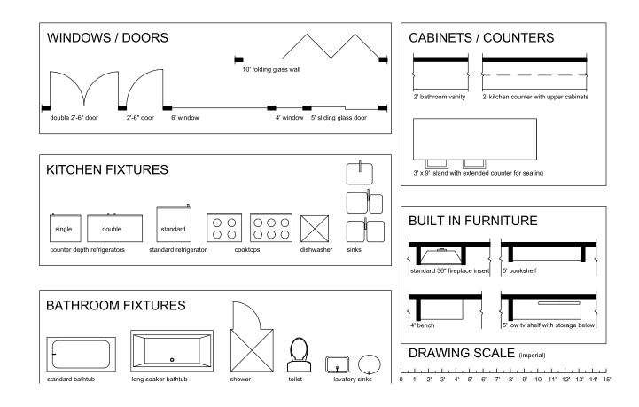
This sheet contains templates of the standard elements of residential construction. They are at the same scale as the plan documents for this project. Use them as a guide when working on the exercise by tracing the required elements into your concept design. Feel free to re-size the length of the windows, built-ins, cabinets and counter elements to suit your specific needs.
