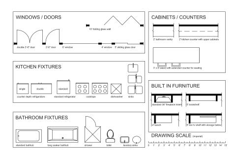
This sheet contains templates of the standard elements of residential construction. They are at the same scale as the plan documents for this project. Use them as a guide when working on the exercise by tracing the required elements into your concept design. Feel free to re-size the length of the windows, built-ins, cabinets and counter elements to suit your specific needs.
